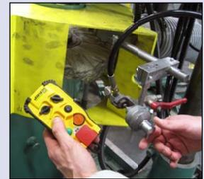
Step by step machine control and setting through the wireless emergency stop system or the wireless enabling handle
