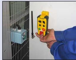
Detection of the wireless emergency stop system or wireless enabling handle on the charger support
